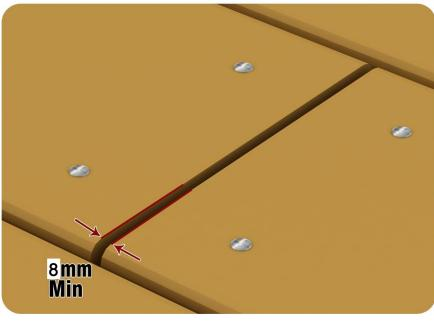
Make sure the reserved expansion joints between two WPC decks at least 8mm.
